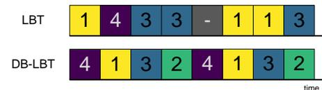
Fig. 1: Exemplary channel access sequence for four contending nodes using LBT (top) and DB-LBT (bottom). Colors and numbers refer to a node’s successful transmission, the dash – to a collision. The sequence for LBT is taken from simulation (Section V). LBT’s random access leads to short-term unfairness and collisions. DB-LBT finds a round-robin transmission schedule that improves fairness and reduces collisions.
